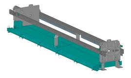
The drip tray, installed between the feet of the machine, is a downward-opening device that, when closed, collects wash water and other drips and discharges via a launder. The drip tray opens completely at the end of the filtration cycle to allow the discharge of the filter cakes.
