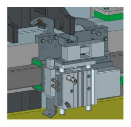
A weight-control and plate-shaking system can be installed on the plate shifting device allowing the machine to operate automatically. This system lifts the plate and measures its weight by means of a load cell. This value is compared with the preset plate weight and, according to this measure, the system decides whether to shake and weigh the plate again or to continue with the plate shifting.
