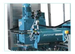
A push-to-close hydraulic jack, controlled by a special hydraulic power unit installed on the machine, performs the closing and sealing of the plate pack. The pressure control system is connected directly to the jack ensuring safe operation.
