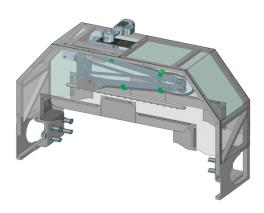
In order to increase the useful life of the filter cloths, the machine can be equipped with a high-pressure cloth washing device. This system will periodically perform a deep cleansing of the cloth to restore its performance characteristics.
