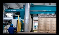
Reliable cloth cleaning using a robotic device ensures that optimum filtration rates are maintained.
