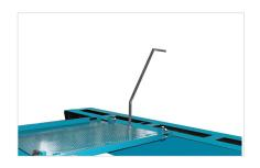
Sliding platform, positioned under the plate pack for inspection and replacement of cloths.
