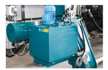
The plate pack closing and opening system delivers high reliability in all working conditions.
