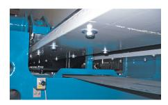
The plate-shifting mechanism, located inside the upper beam, is effectively protected from sludge, dust and corrosive chemicals by a continuous belt of rubber-lined cloth.
