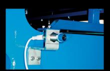
A laser control system ensures correct plate pack alignment and stops the filter press in case of an anomaly, so that any damage can be avoided.
