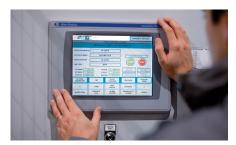
The GHS is provided with a sophisticated automation system equipped with a human-machine interface (HMI) that simplifies the monitoring of the filter operation, enables quick diagnosis of faults and allows the continual adjustment of filtration parameters in order to optimise the process to suit variable feed conditions.
