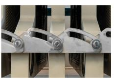
The cake discharge time is significantly reduced compared to traditional plate opening-closing systems with the use of an accordion-style plate pack opening and closing system. This fast operation increases the filter's throughput production.
