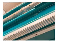
The automatic cloth-shaking device, which is programmed to occur after the plate pack fully opens, ensures the filter cakes are properly discharged and removes possible cake fragments from the cloths. This system, along with the cloth rinsing system, allows the
