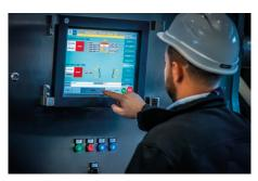
GHT F filter presses are provided with a PLC-based automation system complete with a human-machine interface (HMI) which simplifies monitoring of the filter operation and diagnosis of faults. Additionally, it allows for continuous adjustment of filtration parameters in order to optimize the variable requirements of the process.
