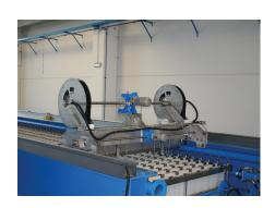
The automatic in-situ cloth washing system, which is programmable according to the user's needs, uses high pressure wash water and directional sprays to effectively regenerate the filter cloth permeability. The results are filter cloths with more consistent filtration performance and longer life.
