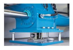
Placed under the supporting feet, load cells constantly monitor the machine weight to ensure all cakes are discharged. The throughput of each load can also be recorded for accurate production tracking.
