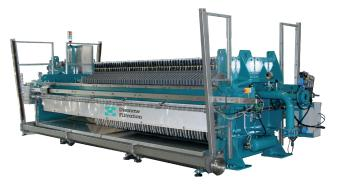
Thanks to its dewatering power and flexible operation, the Diemme® Filtration AUTOMAT filter press achieves the best filtration results in all applications and industries characterised by a limited number of daily filtration cycles, or for the filtration of slow filterability products. ME
