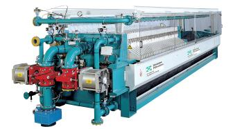
The Diemme® Filtration ME Filter Press is a side beam press which is extremely versatile. Thanks to the simultaneous opening system of the plates pack, the cakes release is extremely quick. For this reason this machine is suitable for high filterability products with high filtration speed.
