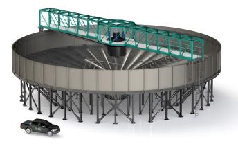
Special care is allocated for bolted-tank modular design, core of our traditional thickening equipment,
