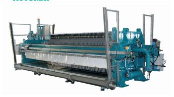
Thanks to its dewatering power and flexible operation, the Diemme® Filtration AUTOMAT filter press achieves the best filtration results in all applications and industries characterised by a limited number of daily filtration cycles, or for the filtration of slow filterability products.
