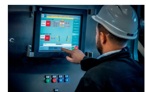
GHT F filter presses are provided with a PLC-based automation system complete with a human-machine interface (HMI) which simplifies monitoring of the filter operation and diagnosis of faults. Additionally, it allows for continuous adjustment of filtration parameters in order to optimize the variable requirements of the process.
