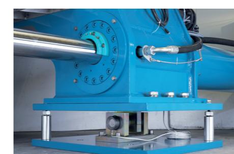
Placed under the supporting feet, load cells constantly monitor the machine weight to ensure all cakes are discharged. The throughput of each load can also be recorded for accurate production tracking.
