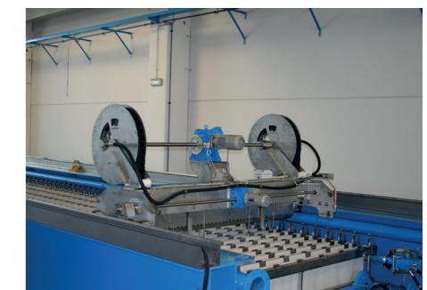
The automatic in-situ cloth washing system, which is programmable according to the user's needs, uses high pressure wash water and directional sprays to effectively regenerate the filter cloth permeability. The results are filter cloths with more consistent filtration performance and longer life.
