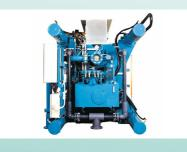
The fixed header is made of a high-tensile steel "cellular" structure in order to best resist stress and it supports 4 hydraulic jacks which are responsible for holding the plate pack closed.
