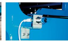
A laser control system ensures correct plate pack alignment and stops the filter press in case of an anomaly, so that any damage can be avoided.
