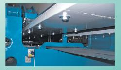
The plate-shifting mechanism, located inside the upper beam, is effectively protected from sludge, dust and corrosive chemicals by a continuous belt of rubber-lined cloth.
