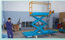
Developed for large machines, the sliding hydraulic platform allows inspection of filtering elements and routine machine maintenance in a convenient, quick and safe way
