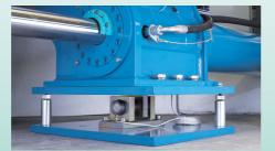
Placed under the supporting feet, load cells constantly monitor the machine weight to ensure all cakes are discharged. The throughput of each load can also be recorded for accurate production tracking.
