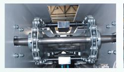
The carousel plate shifting device assures quick and sequential plate movement by means of an automatic transport system controlled by an inverter.
