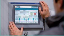
The GHT is provided with a sophisticated automation system equipped with a human-machine interface (HMI) that simplifies the monitoring of the filter operation, enables quick diagnosis of faults and allows the continual adjustment of filtration parameters in order to optimise the process to suit variable feed conditions.
