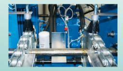
This device ensures the perfect operation of the shifting device, thanks to two brushes that lubricate the carousel chain preventing friction and jams.
