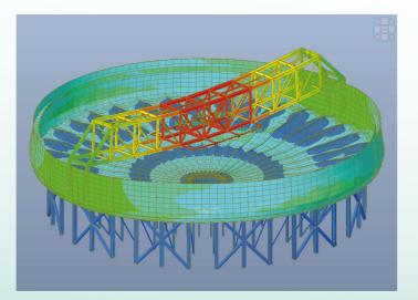
Special care is allocated for bolted-tank modular design, core of our traditional thickening equipment, today optimized for mining industry. Compared with the on-site welded tank, the bolted design allows:
